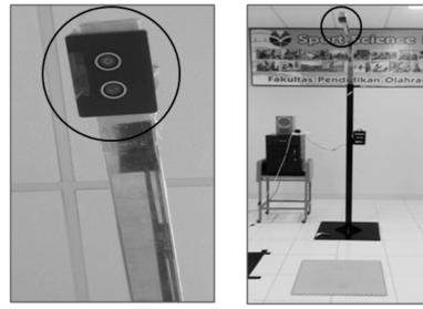
Figure 6. Sensor HC-SR04 ultrasonic
