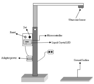
Figure 5. Prototype of leg power device
